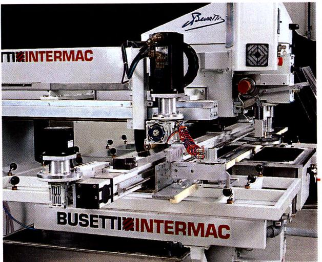
(GB) The glass movement arm allows several holes to be drilled without moving the stops.
