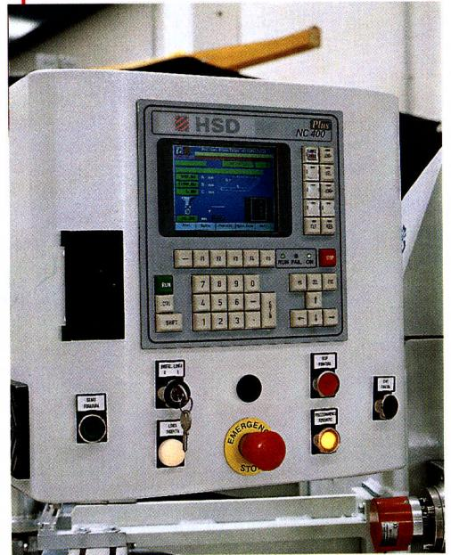
(GB) Intelligent single bit drilling machine programmable from the office. The machine self-learns the material thickness and gauges drill wear.
