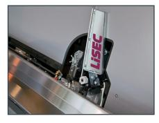
The extended lever supports the frames during the bending process
