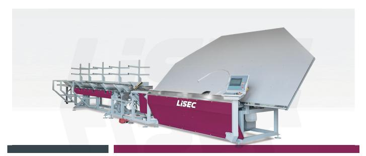
The BSV-45NK is a fully automatic spacer profile bending machine for processing all conventional, synthetic and composite spacer frames for the production of insulating glass.
